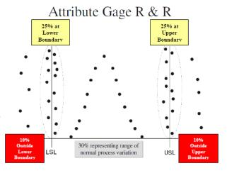
Gage studies should be re-verified at a frequency that is appropriate for gage use and wear. Recommendation - Gage re-verification studies should be completed at the time of calibration
